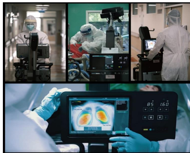
Figure 5. Fujifilm FDR Nano mobile radiodiagnostic device with Fujifilm REiLI AI platform aimed at automatic evaluation of lung images for the purpose of diagnosing multiplicative findings. Immediately after the examination, the AI algorithm provides a graphical and textual warning of a potentially dangerous finding.
